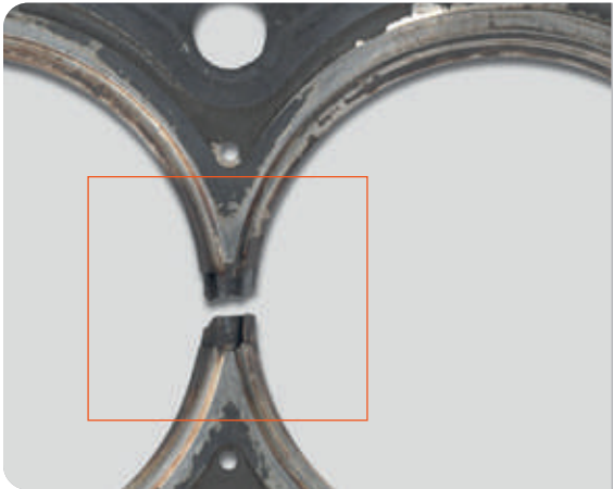
Broken web caused by high component dynamics
