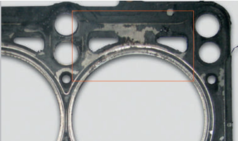
Elastomer coating damaged by overheating
