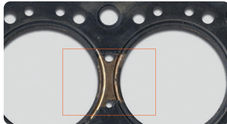
▲ Scorched elastomer coating
