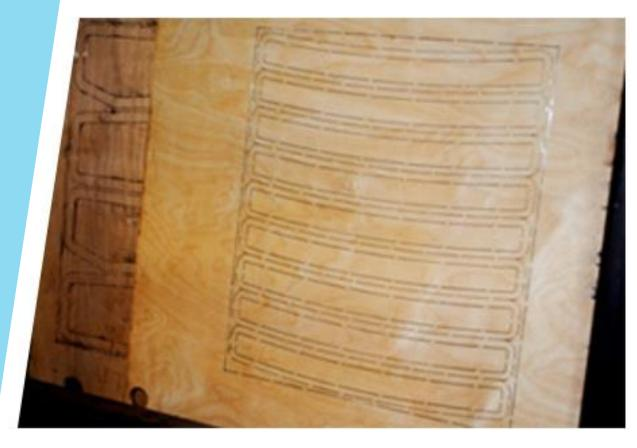
Finished parts are created by compressing the sheets of material underneath razor sharp tools that are made and maintained on-site.
