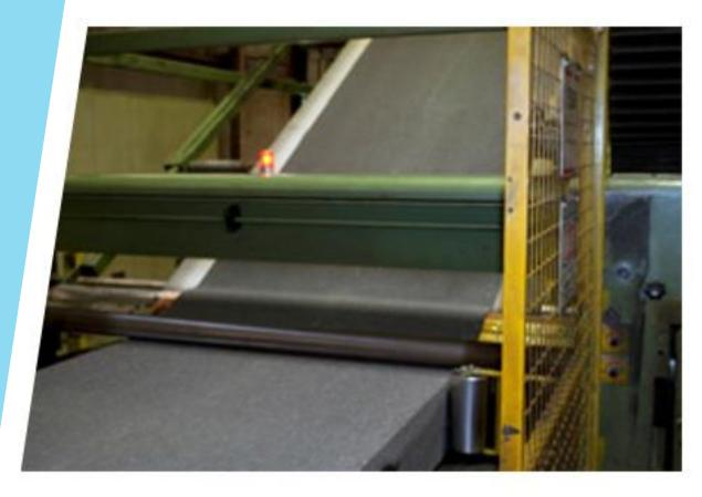
The buns are split into sheets that are the precise thickness of the customer product to be produced.
