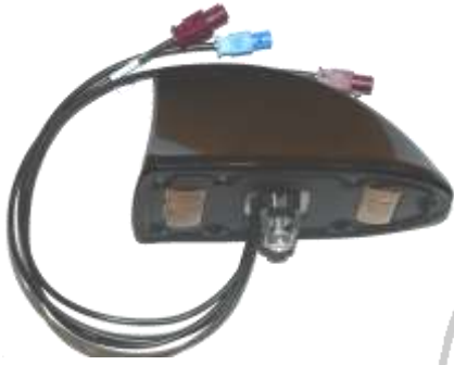
Roof Mount Antenna
