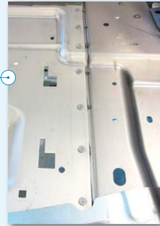
Aluminum parcel shelf joined to steel body in the VW Passat B8 using Flexweld ®
