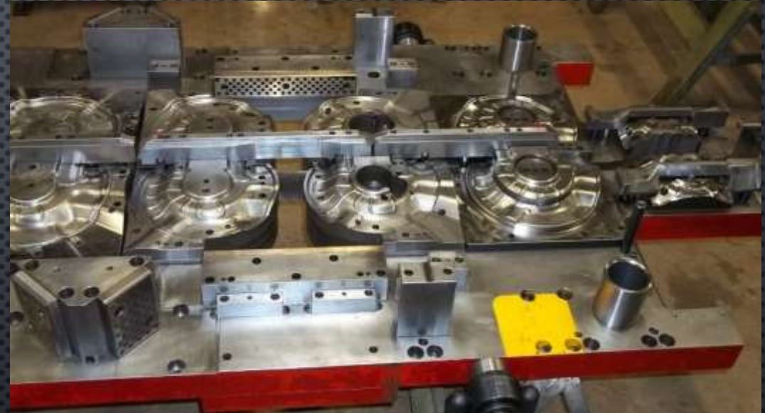
Toyota Brake Shield L/R Progressive Die
