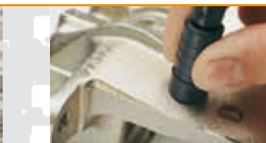
PHASCOPE® PMP10: Zn/Fe with a rough surface
