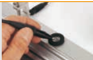
ANOTEST® YMP30-S: Testing the seal of anodised coatings
