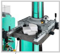
Material compatible: e.g. processing solid silicone (HTV) or moist polyester (BMC) with INJESTER tamping device.
