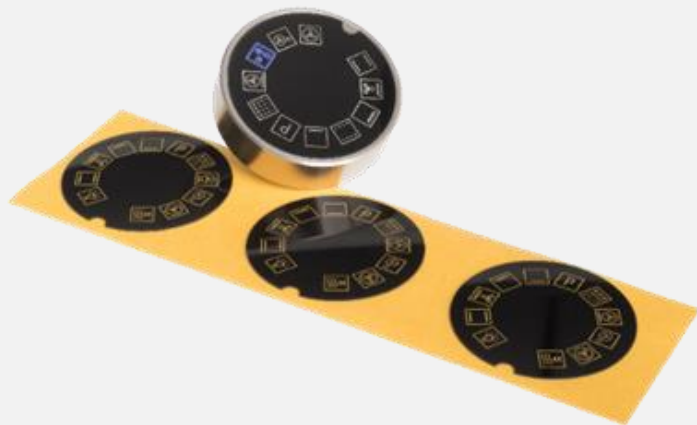
Rotary knob for Oven, Dishwasher or Washing machine. After print on backside material, Lexan is laminated with a transfertape with transparent acrylic adhesive.
