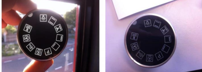
Rotary knob for Oven, Dishwasher or Washing machine. After print on backside material, Lexan is laminated with a transfertape with transparent acrylic adhesive.
