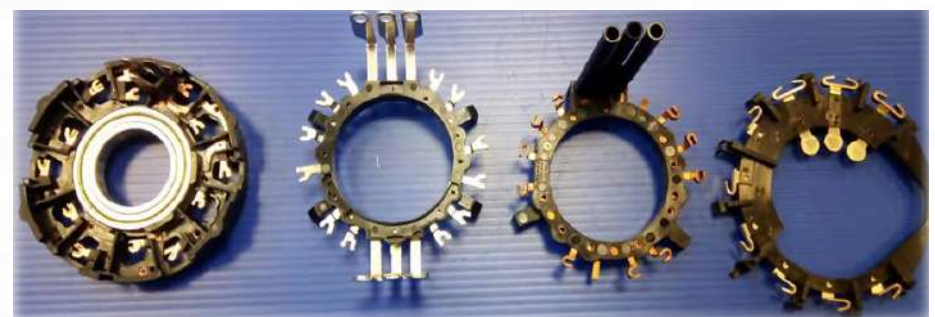
Busbar Assembly Over-Molding
