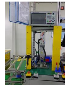
Stator performance test
