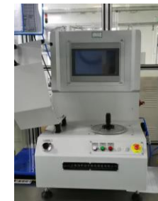
Rotor flux measurement
