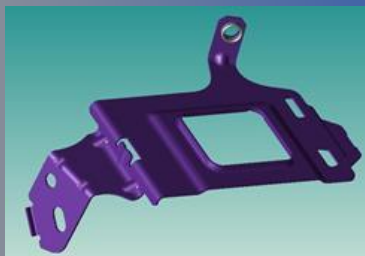
PPAP OK – SOP 2023 68571908AA - CSWM ECU BRKT ASM 23.5 MY VF BEV Process: Stamp + Spacer Weld + Ecoat
