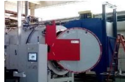
Nitriding Furnace (Payload 2.5 tons)
