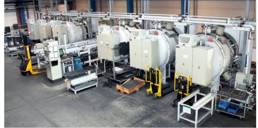
ModulTherm-4 System with individual Vacuum pump sets
