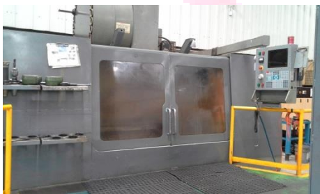
EQUIPMENT: MACHINING CENTER CNC ID: MU-18 CHARACTERISTICS: MODEL VF 6 /50
