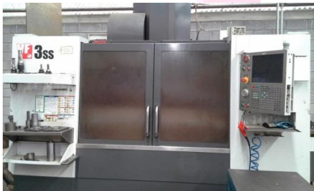
EQUIPMENT: MACHINING CENTER CNC ID: MU-07 CHARACTERISTICS: MODEL VF 3 SS
