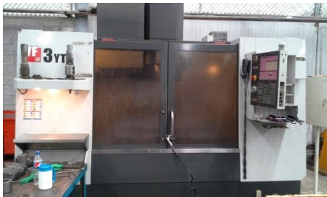
EQUIPMENT: MACHINING CENTER CNC ID: MU-04 CHARACTERISTICS: MODEL VF 3/50 YT
