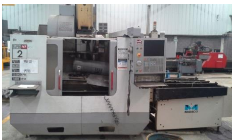
EQUIPMENT: MACHINING CENTER CNC ID: MU-10 CHARACTERISTICS: MODEL VF 2 SS
