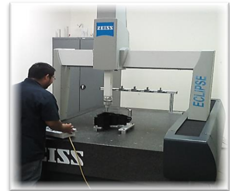
CMM 3D accurate measurements
