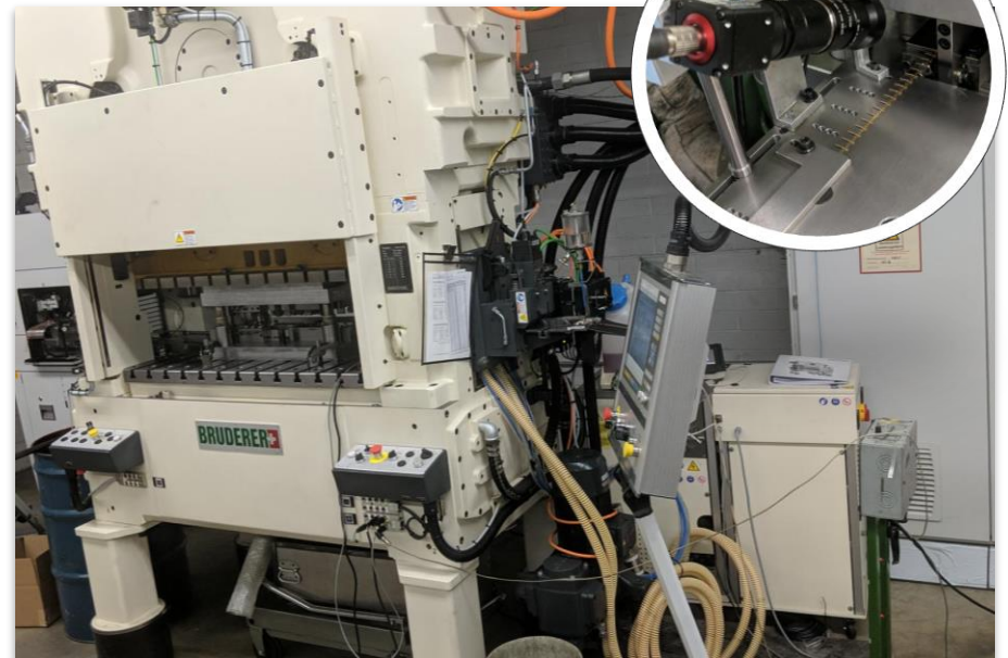
High-Speed Production with Inline Vision Inspection System
