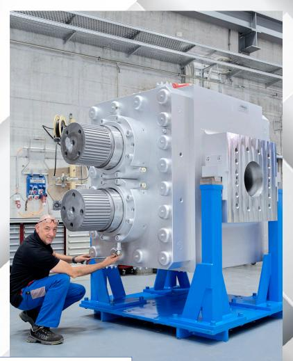
Polyrex gear pumps by MAAG Group are used in compounding applications. They ensure the necessary pressure build-up after an extruder so that the plastics can be cut into plastic pellets in the pelletizer.
