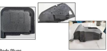
**Body Plugs** Typical materials: PE foam, barrier, fibrous absorbers
