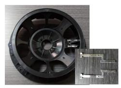
Metal clips for electrical connection over molded in plastic housing
