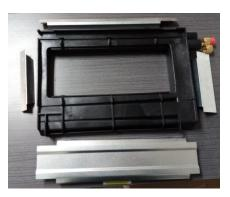
Assembly of metal components to molded plastic parts
