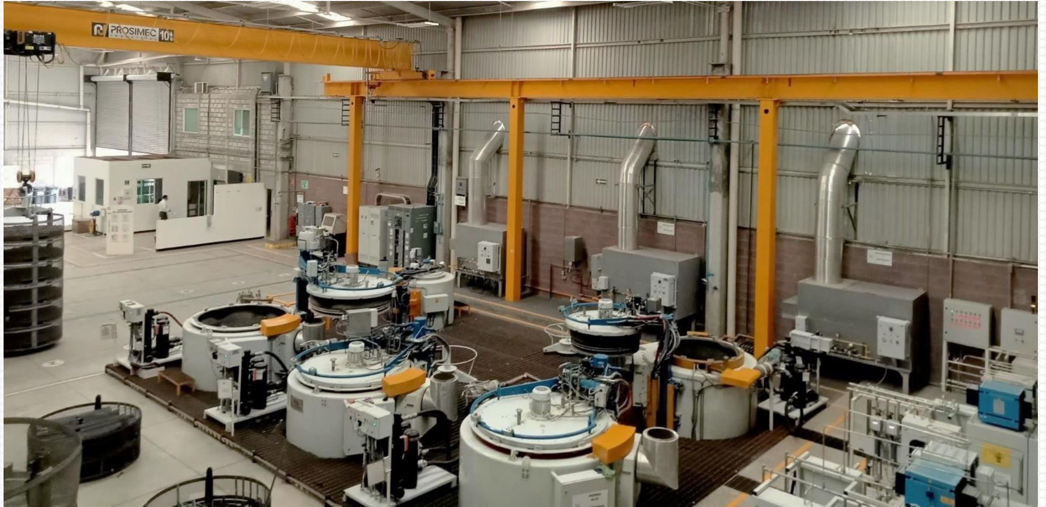
5 Pit Nitriding Systems, fully compliant to SAE2759-12b/10b Gas neutralizers, Gas panels, Inconel baskets, et al.
