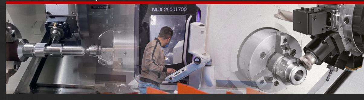
• Machining center (5-axis CNC lathe) with the ability to machine: turning, facing, boring, threading, grooving, drilling, knurling, conical turning, parting off, flattening, among others. With 3" diameter material clamp.
