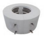
The Fibrothal® GSO heater module has a unique support structure for fixing in tough conditions which contributes to a vastly improved service life and provides power loadings up to 100 kW/m². The module offers high temperature uniformity while being flexible in design.
