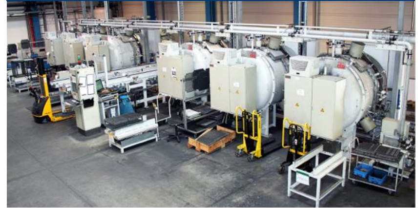
ModulTherm-4 System with individual Vacuum pump sets
