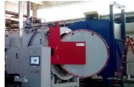
Nitriding Furnace (Payload 2.5 tons)
