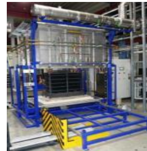
ModulTherm-4 System with individual Vacuum pump sets
