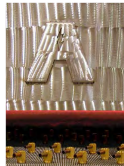
Figure 1. Parts Entering a Continuous Brazing Furnace.
