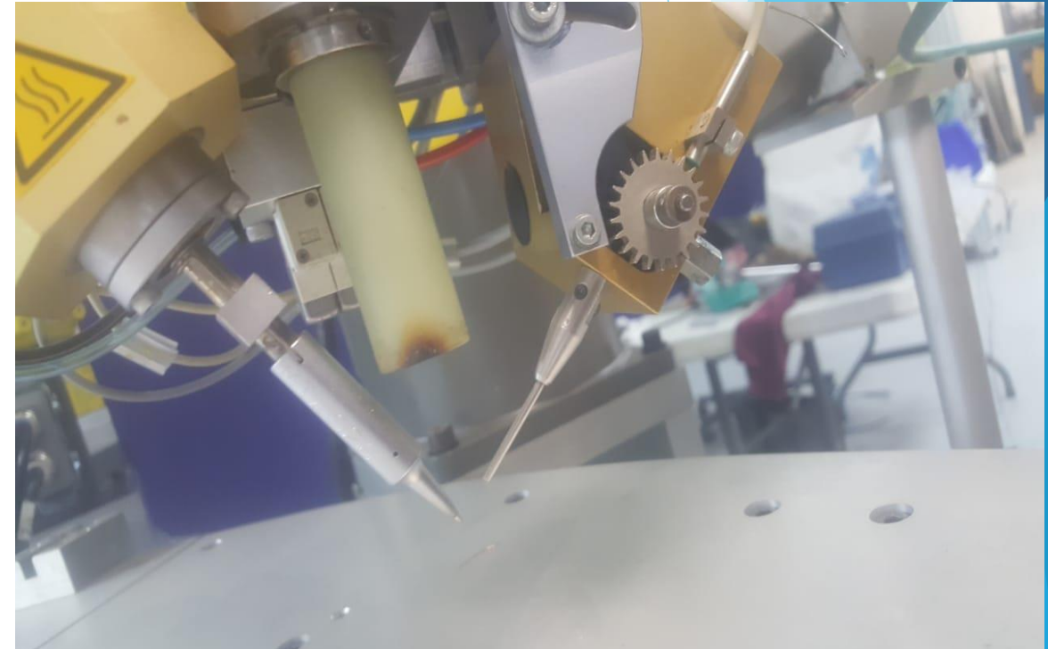
Soldering station whit FANUC ROBOT
