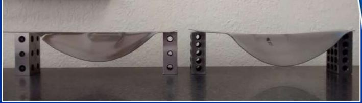
SSAB Strenx 1100 Hit height 57mm FRACTURE MS 1300 Hit height 57mm FRACTURE
