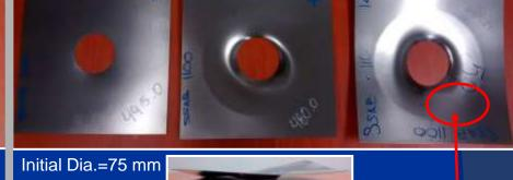
Dia. before fracture= 81.4 mm Large oil can effect approx. 31mm
