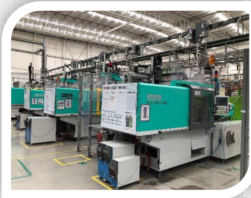
Injection Molding Machines (27 from 70-260 Ton).
