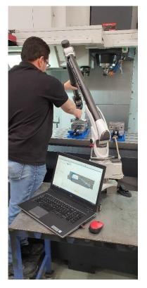
INTEGRATED SCANNER 2019 ARTICULATED ARM COORDINATE MEASUREMENT MACHINE WITH OPTICAL DISTANCE SENSOR MODEL 7725SEI
