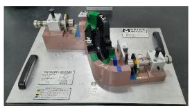
CHECKING FIXTURES: Used for hoses routing inspection.
