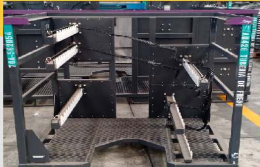
Break Pipes Rack
