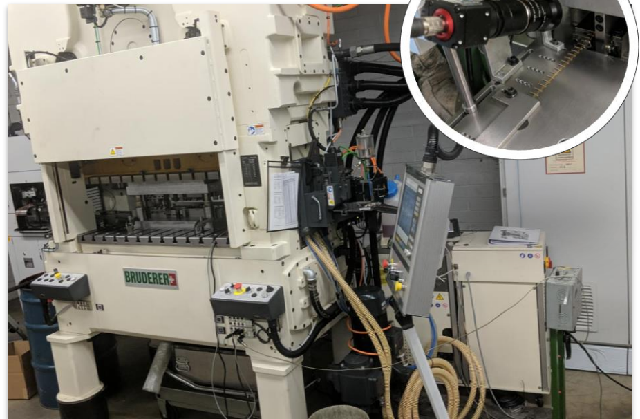
High-Speed Production with Inline Vision Inspection System
