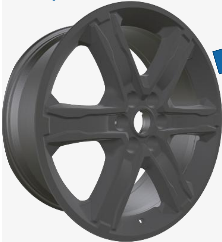
Cast wheel after machining, before painting
