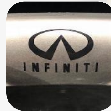
Etch through paint to primer surface- logo
