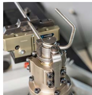
▲ Standard bending tool combines draw and roll bending
