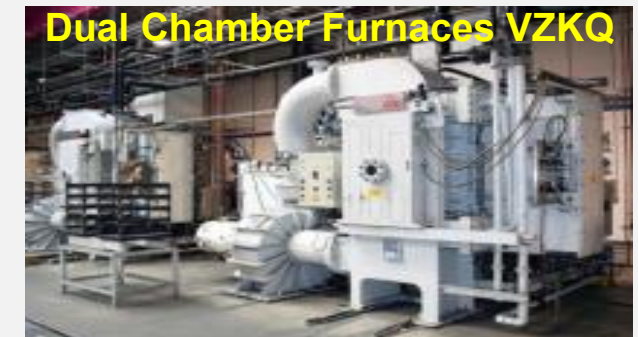
De-Oiling Furnace (for PM Parts)
