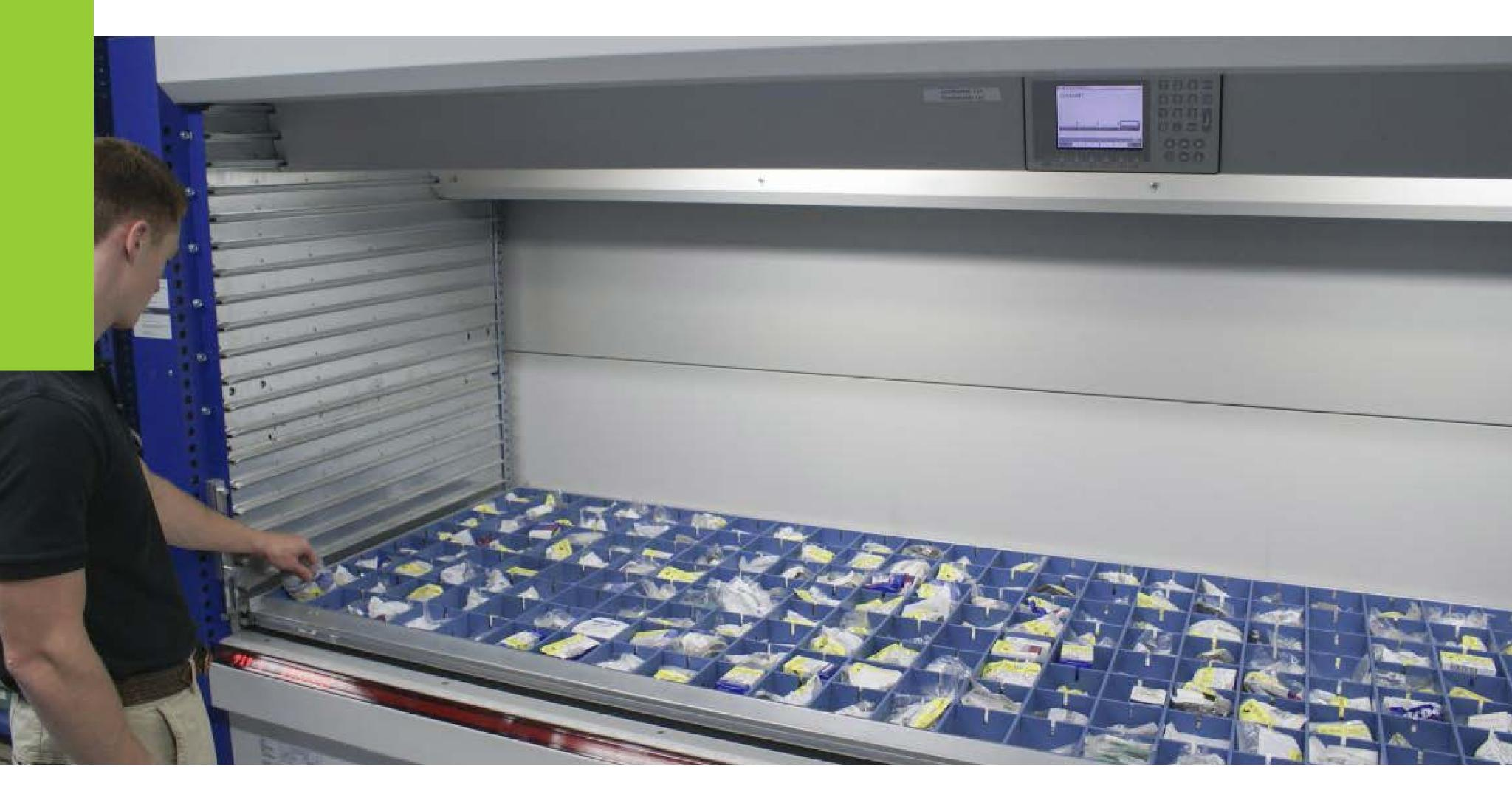
This automatic system allows to select the assortment of items and small parts from containers, cartoon boxes or trays. It is also based in "Good to person" principles, providing a higher productivity in picking operations.
