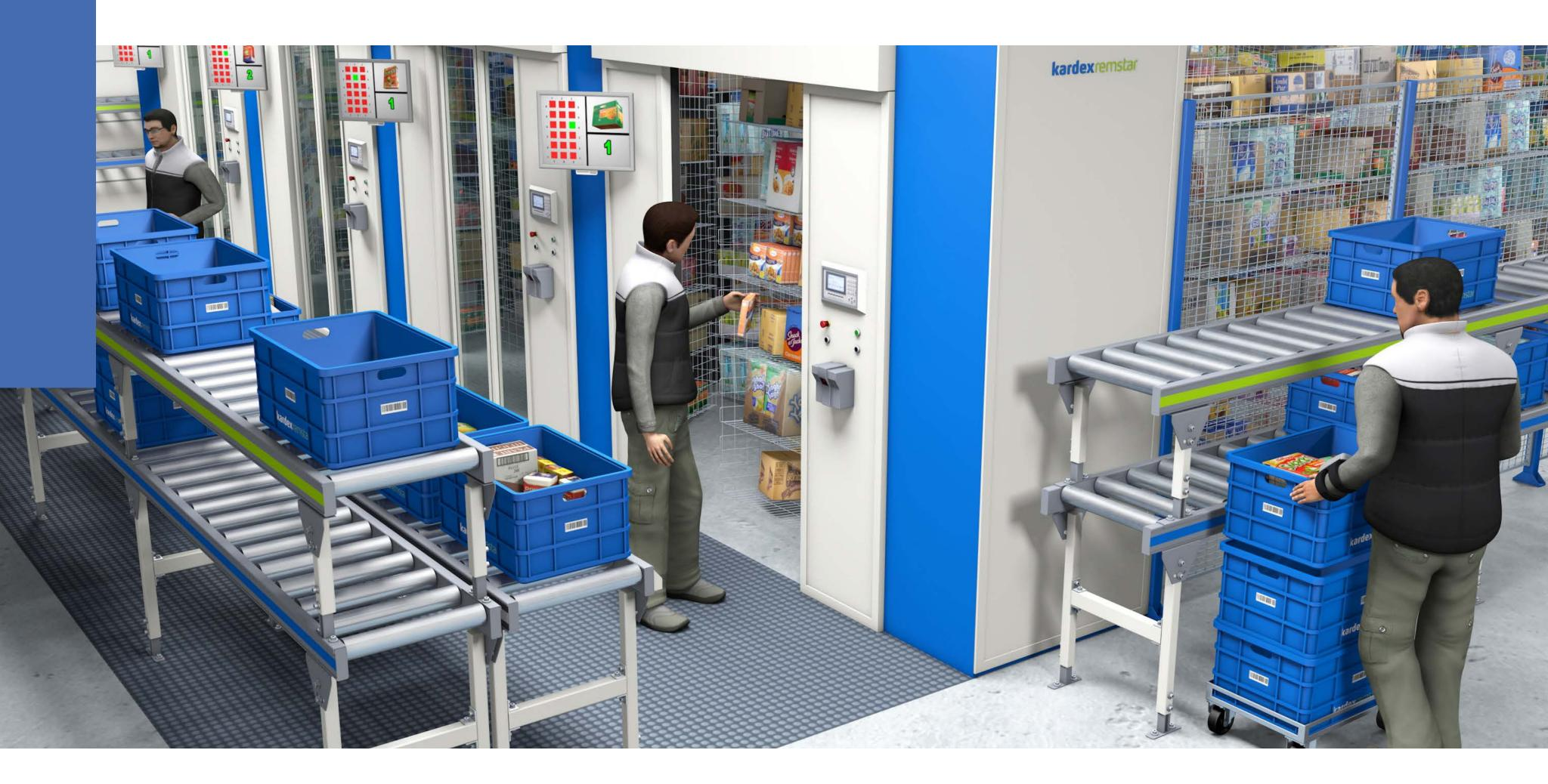
This kind of system **is used** in places where **storage must be safe, profitable,** and quick. The following elements constitute horizontal carrousels:
