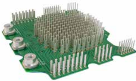
Power Distribution Module
