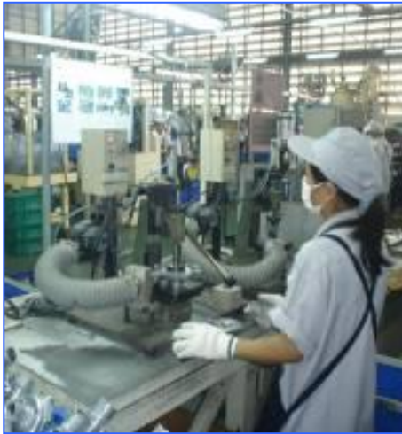
Compressor Part, Shrinkage Fitting
