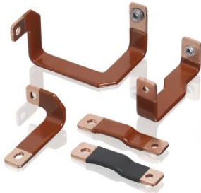
Copper busbars with Dielectric insulated materials (epoxy powder coating and heat shrink tubing) with PEMnut fasteners
