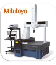
CMM MITUTOYO BRAND MODEL: CRYSTAL PLUS 776 TECH SPECS: (X) AXIS: 700 mm, (Y) AXIS:700 mm y (Z) AXIS:600 mm. RESOLUTION: 0.0001 mm. SOFTWARE: M COSMO BASIC
