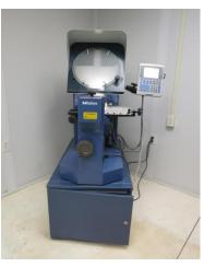
MITUTOYO BRAND OPTICAL COMPARATOR MODEL: PH-A-14 TECH SPECS: (X) AXIS:200 mm, (Y) AXIS: 100 mm RESOLUTION: 0.0001 mm PROJECTION: 10 lenses
