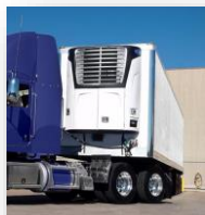
Transportation refrigeration units (TRUs)
