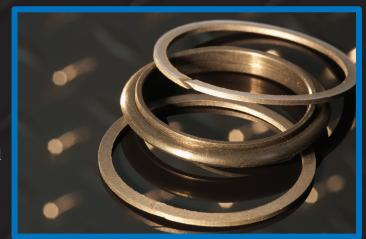
Since inception Aero Brake has been providing quality parts at superior prices to customers across the globe. Our phenolic brake insulators have flown on military aircraft in the Middle-East, our wheel seal packings have traversed Europe on EASA aircraft, and our piston seals (pictured) have kept U.S. domestic transport aircraft on time and under budget.
