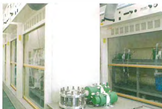
Product testing laboratory for compatibility with semiconductor/liquid crystal display production equipment Equipped with a neutralizing system, this laboratory tests the resistance of Pillar products against various kinds of chemicals for semiconductor production.
