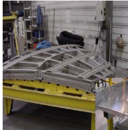
Ground Antenna Sub-Assy
