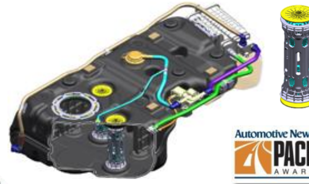
Hybrid Electric Vehicle Pressure Resistant / Slosh Minimization Fuel Tanks w/ Tank Advance Process Technology (TAPT)
