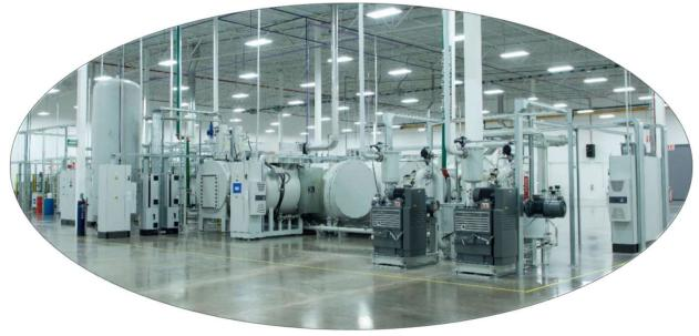
Quench cell is capable of 20 bar gas quench with variable speed fan control
