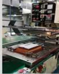
Hot Stamping Machine Up-Down Type 300*150mm
