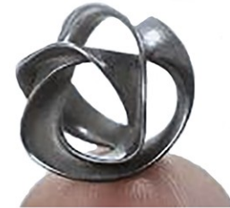
Ames-Additive® MJB Binder Jetting technology
